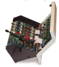
The Console operates from 12 Volts DC, which is available from Zetron's universal power-supply that accepts any voltage from 95 to 250 VAC at 47 to 440 Hz. The universal power-supply has UL, CSA and VDE approvals.
